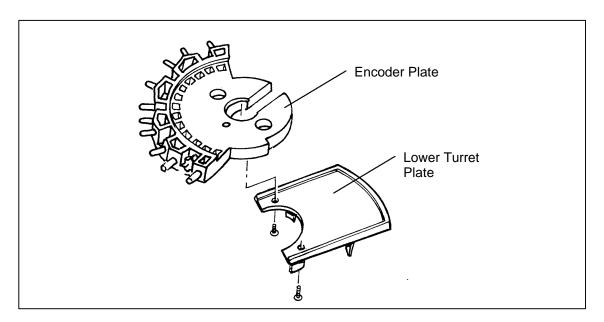
Figure 5-12 Encoder Plate and Lower Turret Plate
